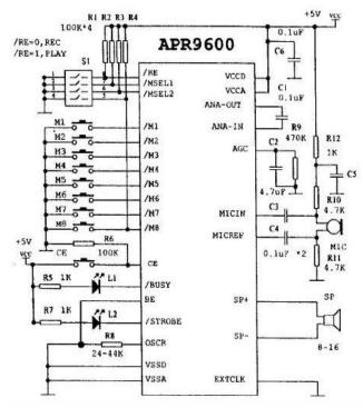
Figure1: circuit diagram of voice module
