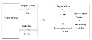
Figure2: architecture of PIC microcontroller
