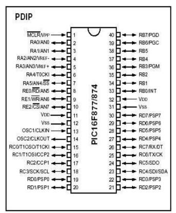
Figure3: pin diagram for PIC16F877
